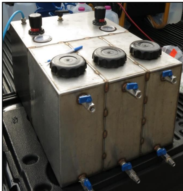
Figure 12. Dry-fog technology apparatus
