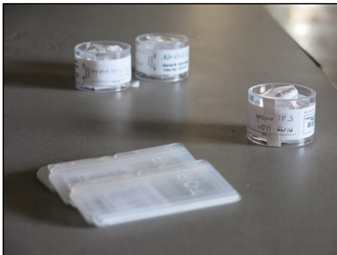
Figure 10. Air and surface sampling equipment
