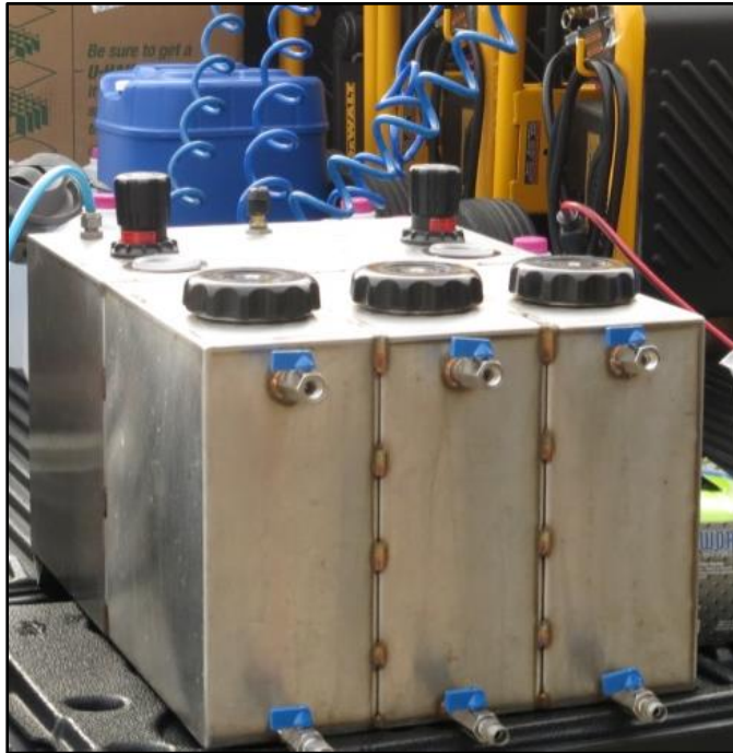
Figure 1. Dry-fog application system
